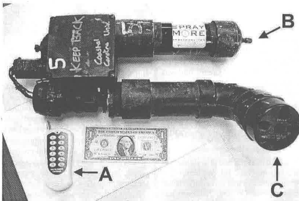
Fig. 1. A Spraymore Mega paintball land mine (with modifications for waterproofing). A: multi-channel electronic trigger; B: Schrader valve for filling with pressurized gas; C: Spray nozzle.
