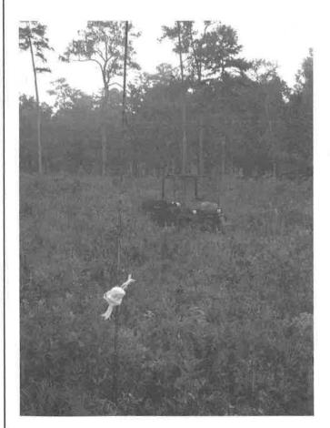
Fig. 3. Off-road vehicle with base poles attached to the front frame. Another base pole is attached to the tailgate but is not deployed in this picture. The white object in the seat is a CD player, and the plastic grocery bag used to store nets is wrapped around the front net pole in this picture.
