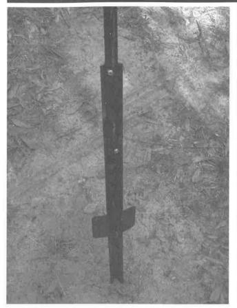
Fig. 1. Base pole showing painted conduit attached to a fence post using mechanical screws.
