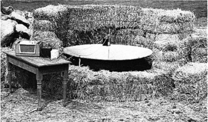
FIG. 1. Equipment used for flight-call detection of nocturnal migrants. From left: recorder, recorder timer, high-pass filter; parabolic reflector surrounded by straw sound baffle, and pre-amplifier with speaker (black box).
