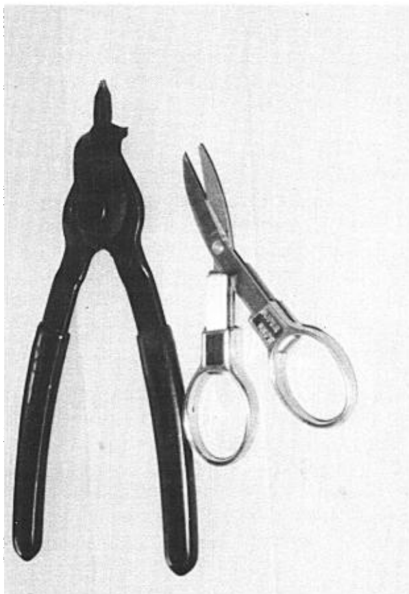
Figure 1. Retaining ring pliers (left) and small scissors. (photo by Gordon E. Howard)
