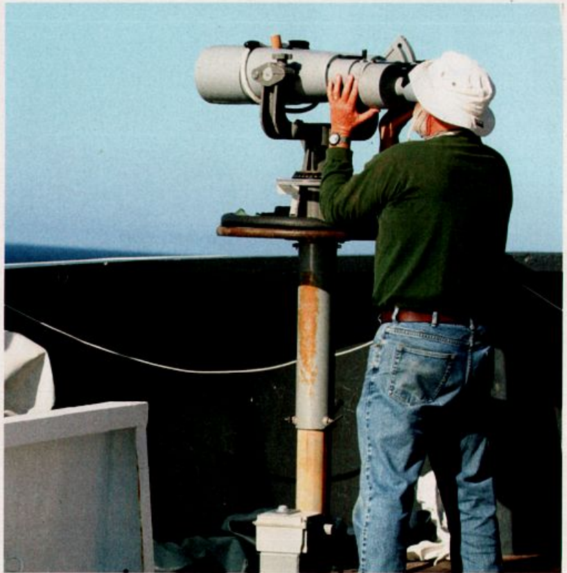
Figure 6. Gary Friedrichsen with 25 x 150 mounted binoculars used by marine mammal and seabird surveyors aboard NOAA vessels. Aptly referred to as "big eyes," these binoculars seem to result in 2–3 times the power and illumination of a single 25x telescope, allowing the identification of mammals up to 9 km (5 nmi) away and birds up to 3.7 km (2 nmi) away. Photograph by Peter Pyle © PRD, SWFSC.
