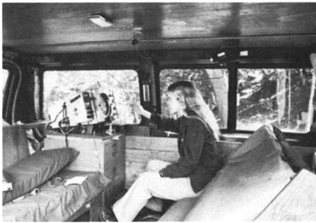
Figure 4. Mobile radar used for investigations. L. Sheriff at the radar console records data manually. Transceiver mounted on the roof is a modified marine radar unit.
