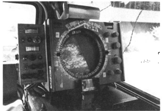
Figure 5. Display console of the mobile radar. Controls at right modify the display. Those at the left of console change output of the radar transmitter. Reflections on the screen are not present during nocturnal observation.
