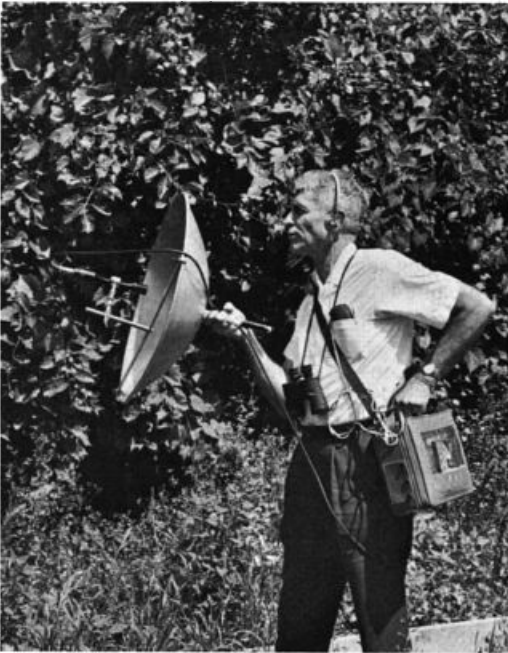
The author in the field, equipped with tape recorder and parabolic reflector microphone.
