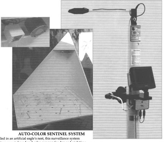
Installed in an artificial eagle's nest, this surveillance system combines near-infrared and color cameras for day and nighttime recording.
