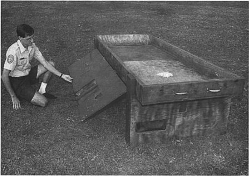
Figure 1. The trough-blind, illustrating basic construction materials, hinged side, and arm holes for grabbing the bird's leg.
