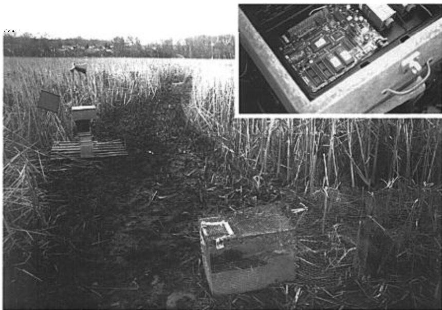
FIGURE 1. Winter photo of trap line in tidal marsh showing walk-in traps with drift fencing running between the traps (top and bottom center), and sound system with solar panel and speaker (upper left). (inset) Digital playback equipment including amplifier, microchip message repeaters (near center) and timing units (upper right) in weather-proof housing.
