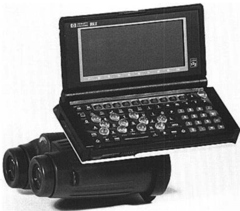
FIGURE 1. Palmtop computer on mounting bracket affixed to a pair of Leica 10 × 42 Ultra binoculars.
