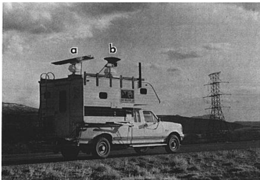
FIGURE 1. The mobile radar lab: a. surveillance radar, b. vertical radar.
