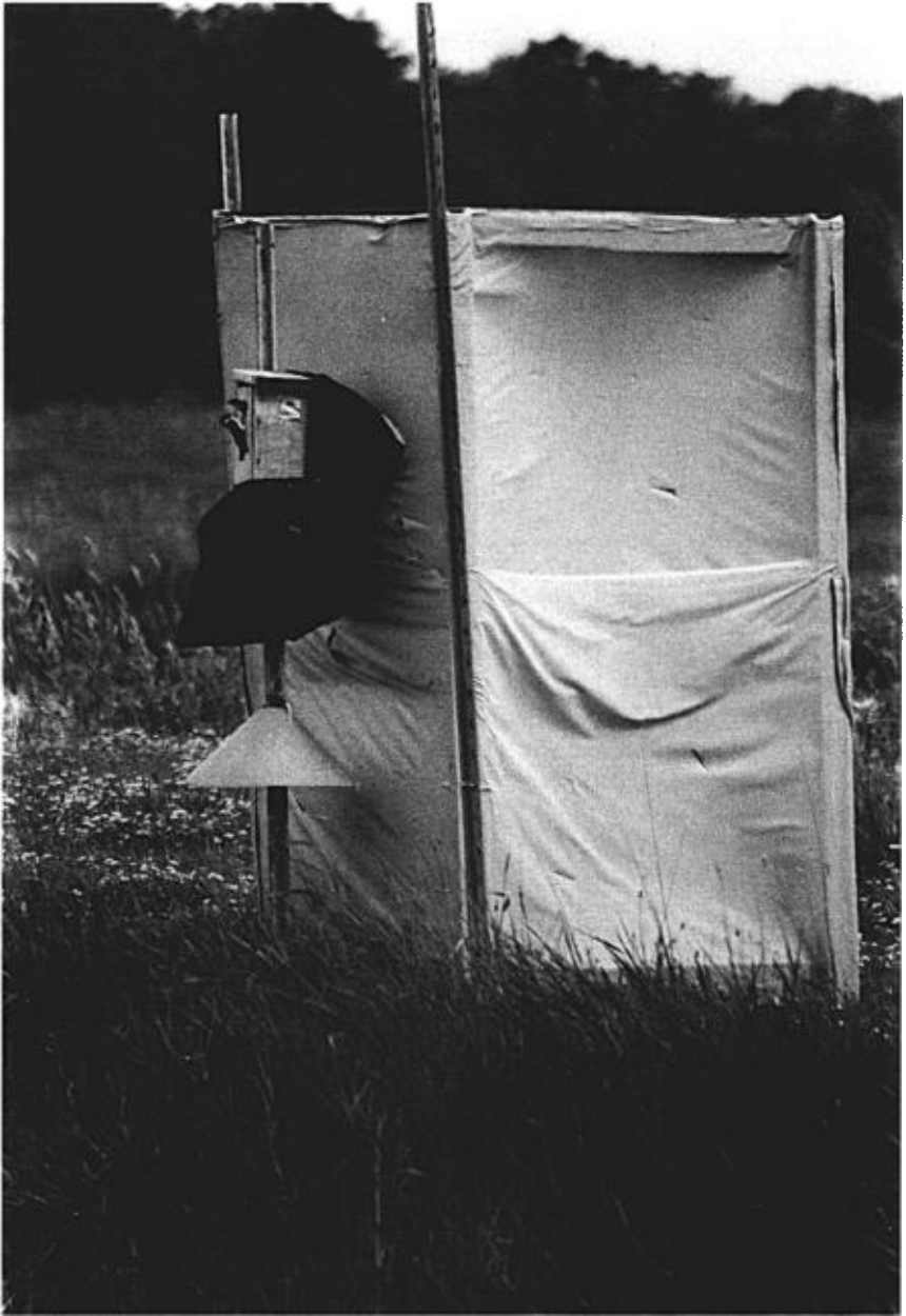
FIGURE 2. Puppet blind and modified nest box. Note the sleeves running between the blind and the nest box for viewing the nest (top) and concealing the puppeteer's arm (bottom).
