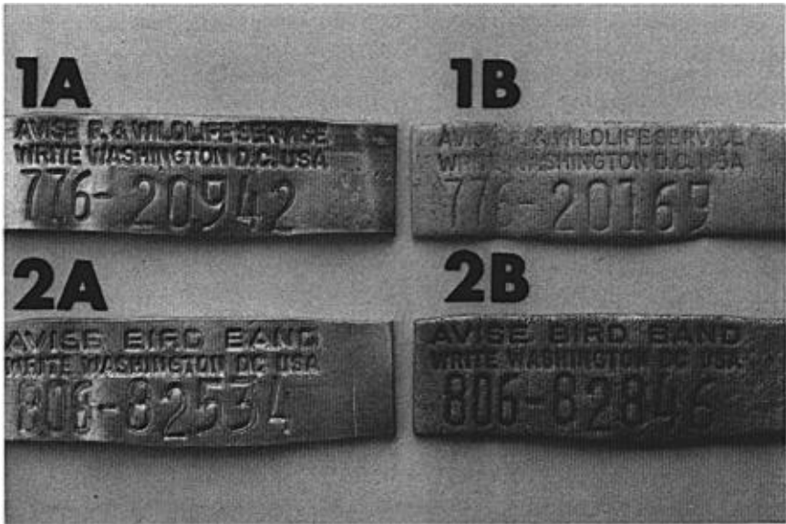
FIGURE 2. New (1A, 2A) and used (1B, 2B) 776 and 806 series butt-end Al bands. The used 776 band had been worn by a Farallon Western Gull for 8.0 years (wt. = 0.59 g), the used 806 band 4.3 years (wt. = 0.69 g).
