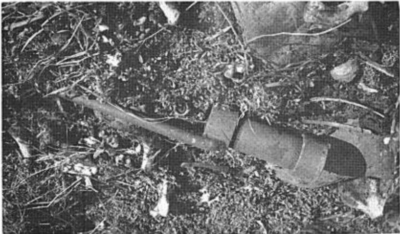
Figure 1. CTI Recoilless Net Trap Cannon (rocket) used to project nets in 1966.
