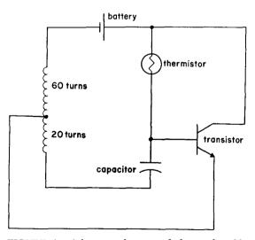
FIGURE 1. Schematic diagram of the implantable temperature transmitter. Various components were tried in the circuit. Those parts listed were found to be most reliable and easily obtained: wire—40gauge copper magnet wire (frequency depends on number of turns in coil); battery—1.4 volt (Mallory 212); thermistor—1000 kohm (Fenwal GABIJI); transistor—NPN (GE D26Er); capacitor—0.68 to 0.1  $\mu$ F tantalum (Allied 162D); encapsulated in Silastic<sup>®</sup>.
