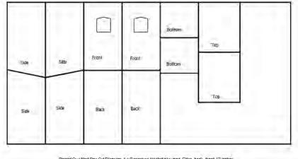
Barned Own Nest Box Cut Diagram. 4 x 8 pressure intelled blywood. Sides, back, front 13 inches wide. Sides 24.25 inches in back, 23.75 inches in from: Bottoms 12 x 13 inches. Tops 14 x 17 inches Entrance hole is 7 x 7 inches, Bottom of hole is 13 inches above bottom of the front place 1.25 inch syare ballsters in literior commer to screev plywood to
