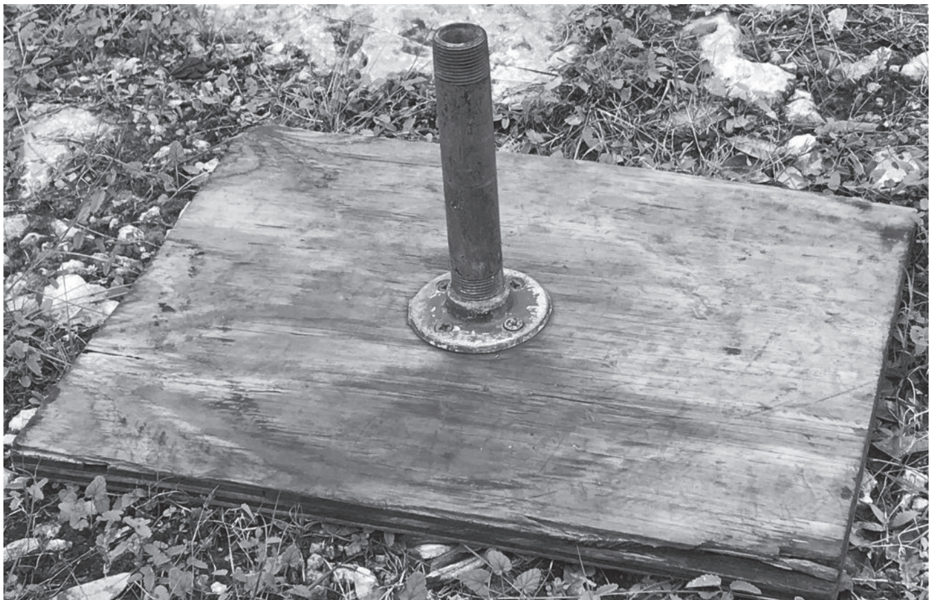
Figure 1. A base constructed from plywood, a flange, and metal pipe nipple for supporting a net pole.
