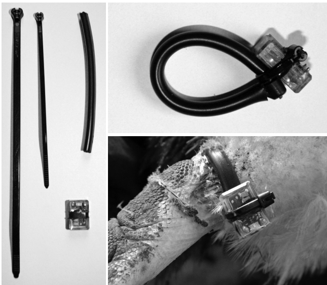
Fig. 1. Photographs of the components required to make the band (left), a completed band (top right) and a band fitted to a wild Southern Rockhopper Penguin on Beauchêne Island, Falkland Islands, that was subsequently released and then recovered unharmed nine months later (bottom right).
