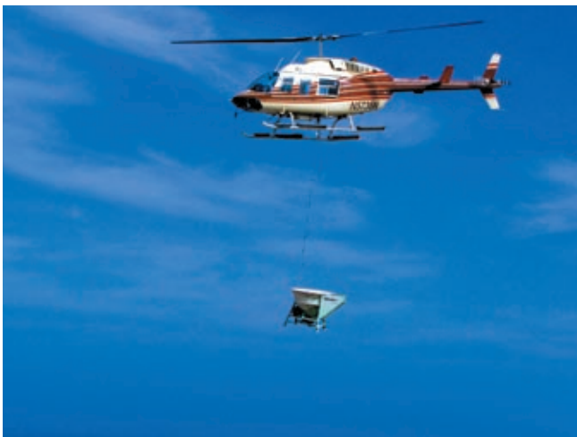
Fig. 6. Aerial rodenticide is dispersed using a modified agricultural fertilizer spreader bucket carried by a helicopter, navigating by a differential global positioning system. Photo courtesy of Island Conservation. See new photo.
