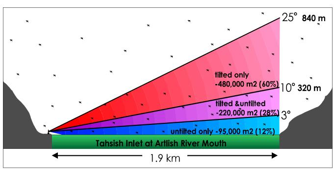
Fig. 3. Cross-sectional representation of exclusive and overlapping scanning areas of tilted and untilted radar units.
