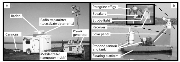
Fig. 1. The BirdAvert (Peregrine Systems, Salt Lake City, Utah, USA) on-demand radar-activated system.
