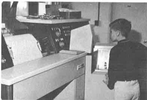
14. Improved Efficiency Through Automation. The introduction of this Univac machine now does in 8 hours what previously have required 800 days to accomplish - program, recover data and print out. Chris Jr. has just moved the key punch and sorting room (on his left) to the Univac Print Out.
