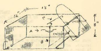
To make it get a piece of  $\frac{1}{2}$ " mesh galvanized hardware cloth, 18 inches wide and 28 inches long. Bend this as the measurements show to form the sides and top. Remember that the selvage end will be the front of the trap. The trap door hinges on this selvage and if such is not available then it would be advisable to reinforce this open end with a piece of #12 gauge wire. Carry this reinforcing wire across the bottom of the trap keeping it four inches from the front as shown.
