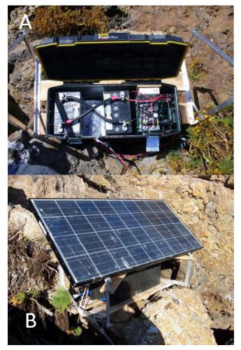
**Fig. 6:** Vocalization broadcast system on Orizaba Rock, 2011: (A) tote box containing MP3 player and other equipment and (B) close-up of solar panel and tote box (photos by L. Harvey).
